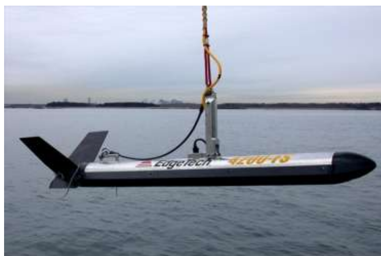
Figure 9. Deployment of Edgetech 4200 Tow fish (Source: MDM)
