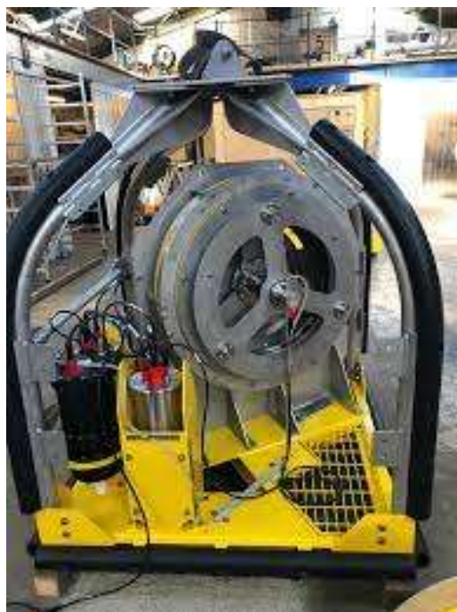
Figure 13. Neptune 3000 CPT rig (Source: MDM)
