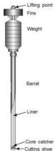
Figure 14. Gravity Corer schematic
