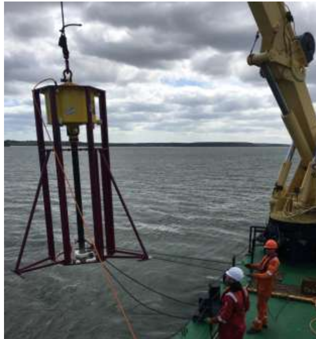
Figure 15. Deployment of Vibrocorer from Survey Vessel (Source: MDM)
