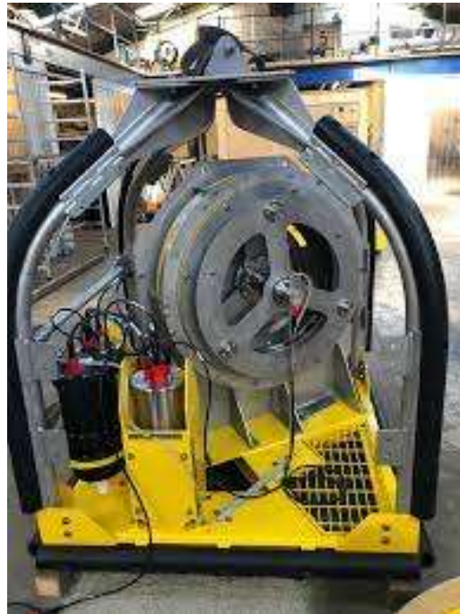
Figure 13. Neptune 3000 CPT rig (Source: MDM)
