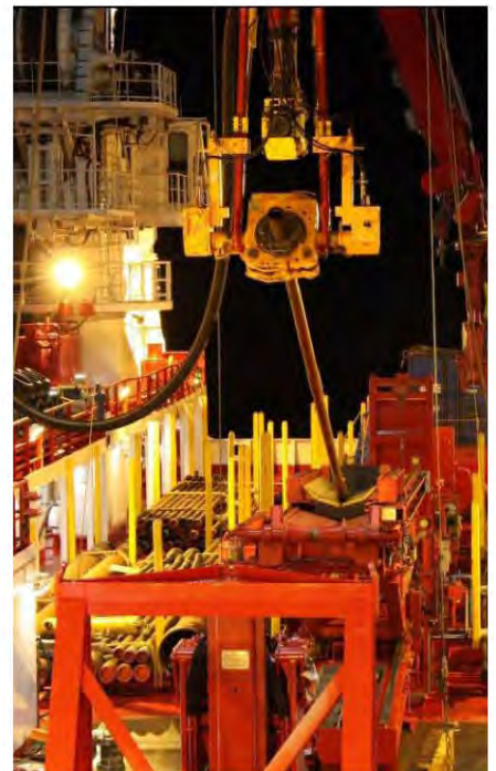
Lifting pipe on the drill deck.
