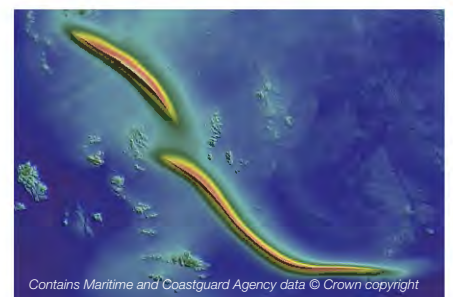
Shaded Relief Bathymetry showing Sandwave detail.
