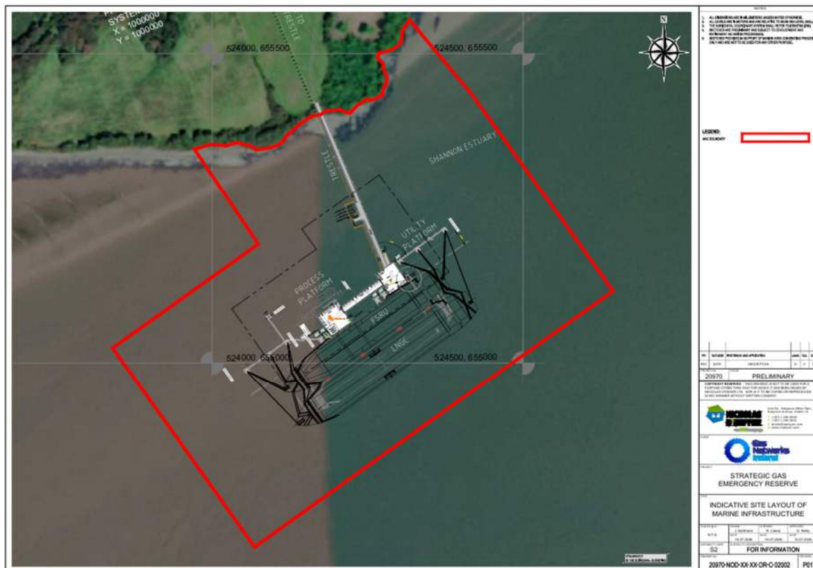
Figure 1 – Applicant Indicative site layout drawing of marine infrastructure and proposed MAC area
