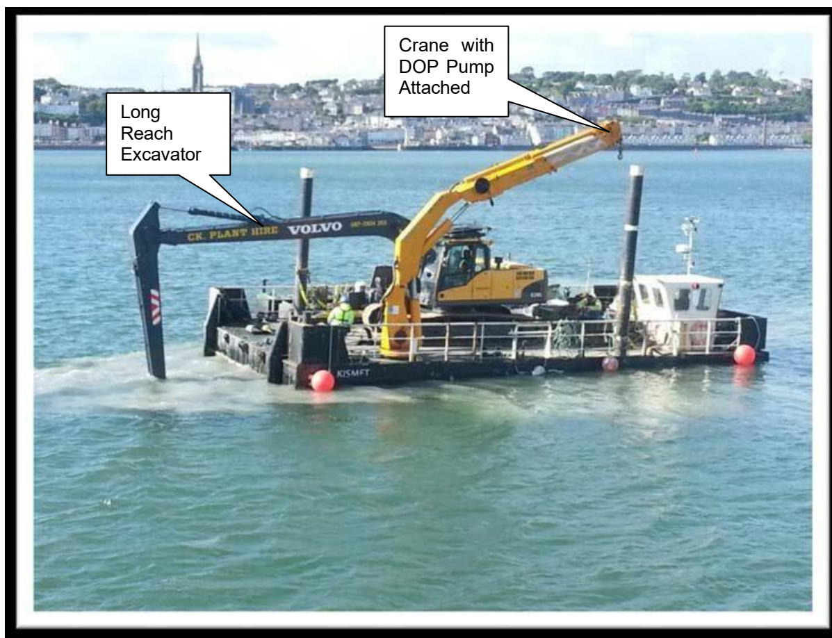
Figure 3 – Typical crane on a 4 unit pontoon raft
