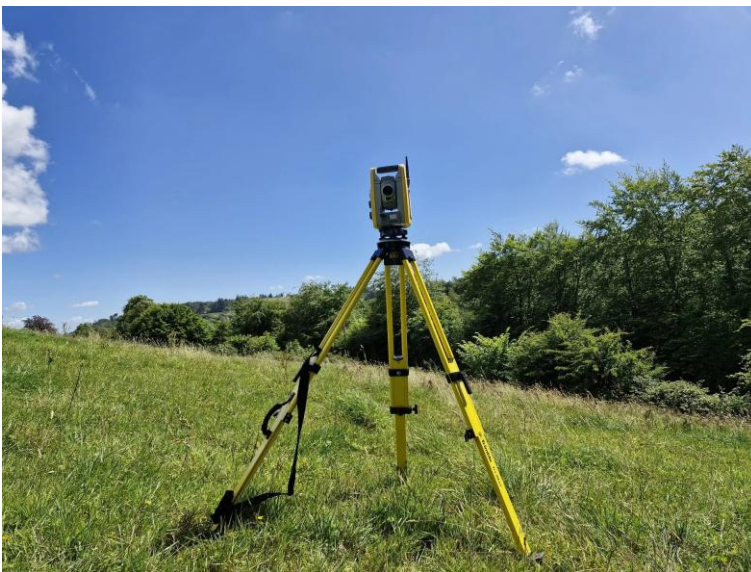
Figure 2-3: Total station set up on a tripod operating as a base station for survey control
