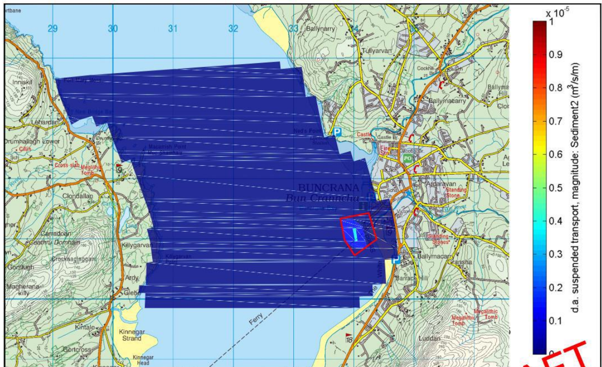
Figure 7.6 Scenario 3 Maximum Suspended Sediment Transport (Instantaneous) (extract from Malachy Walsh and Partners, 2016).
