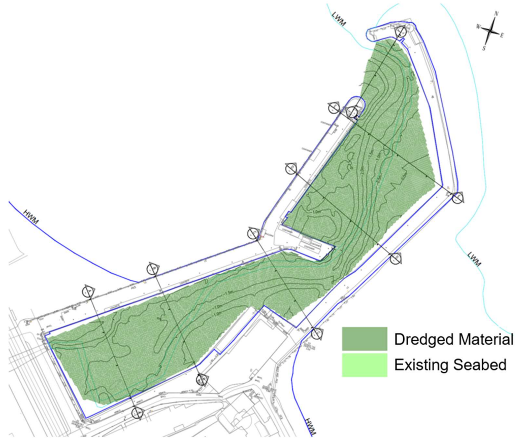
Figure 4-6: -3.0m ODM Dredge Layout
