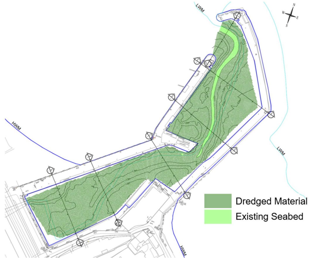
Figure 4-5: -2.0m ODM Dredge Layout
