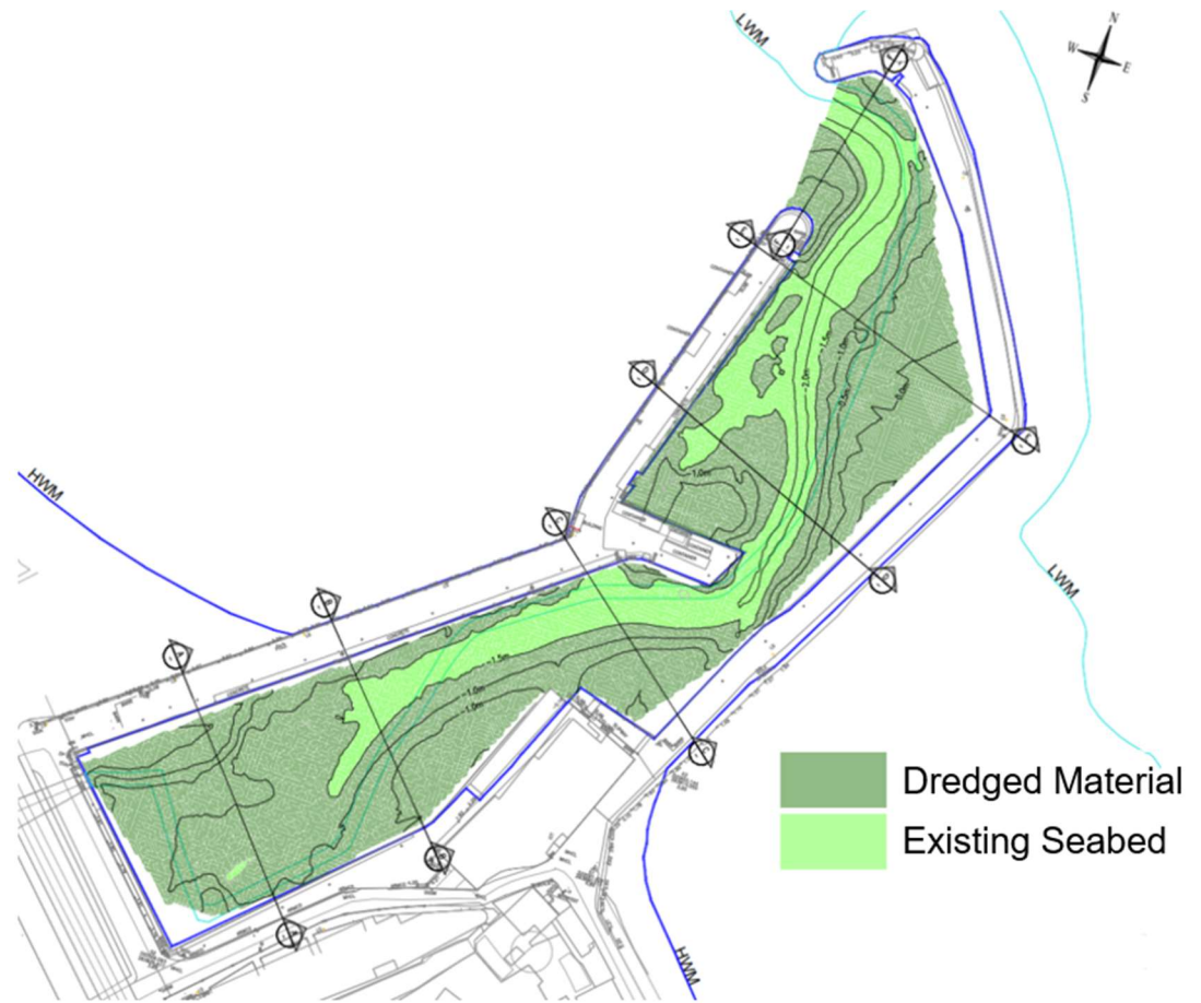
Figure 4-4: -1.5m ODM Dredge Layout
