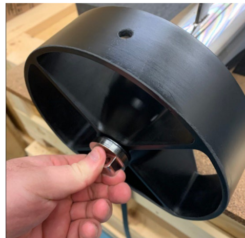
Figure 3-10: Tail Assembly Bolt Installation
