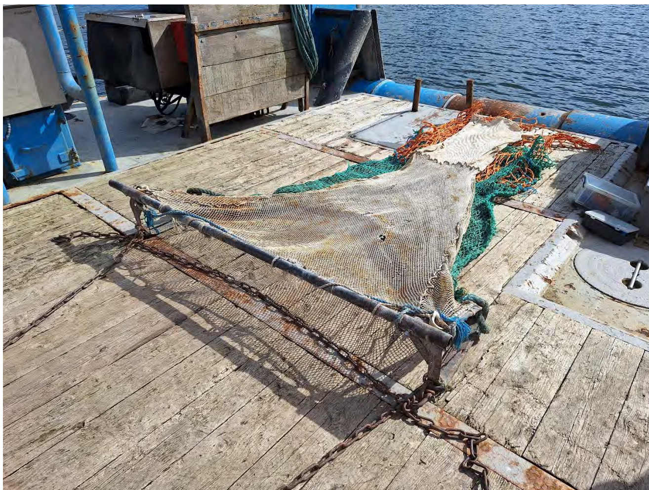
Figure 2-1: Beam trawl (2 m diameter with an 11 mm mesh) on the deck of the Denis Murphy.
