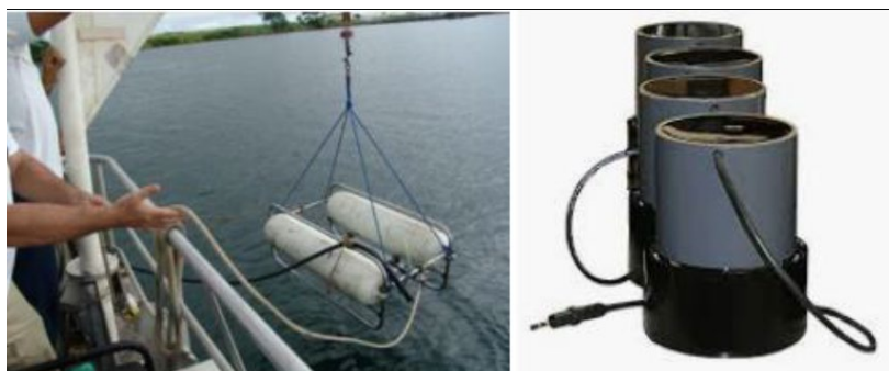
Figure 2-7 Left - Applied Acoustics AA300 being deployed & Right - Typical Hull Mounted SBP - Edgetech 3300
