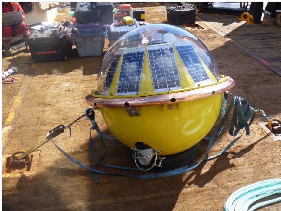
Figure 23: Triaxys wave and current buoy with mounted current profiler on underside.
