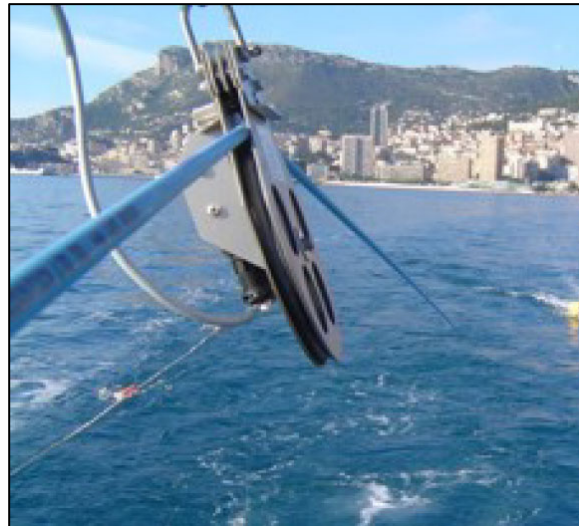
Figure 4: counting pulley for winch-towed C-Max CM2 SSS
