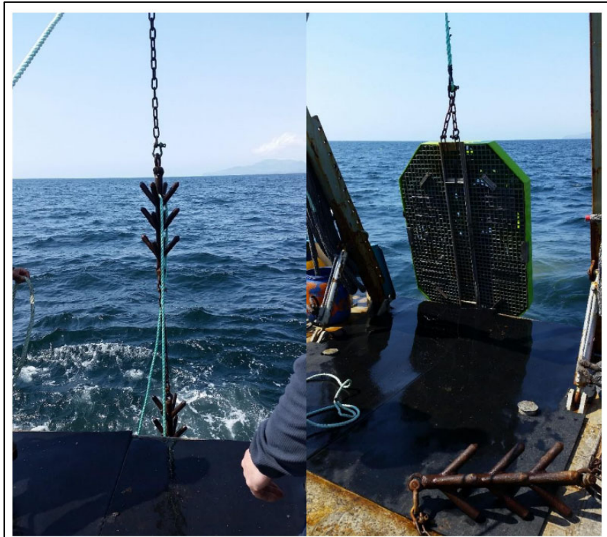
Figure 21 Left – The grapple hook caught with the grapple line; Right – The floating grapple line is winched into retrieve the ADCP frame (Techworks Marine Ltd.)
