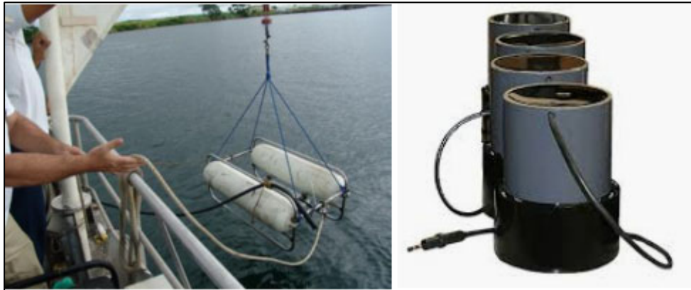
Figure 5: Left - Applied Acoustics AA300 being deployed & Right - Typical Hull Mounted SBP - Seatronics Edgetech 3300
