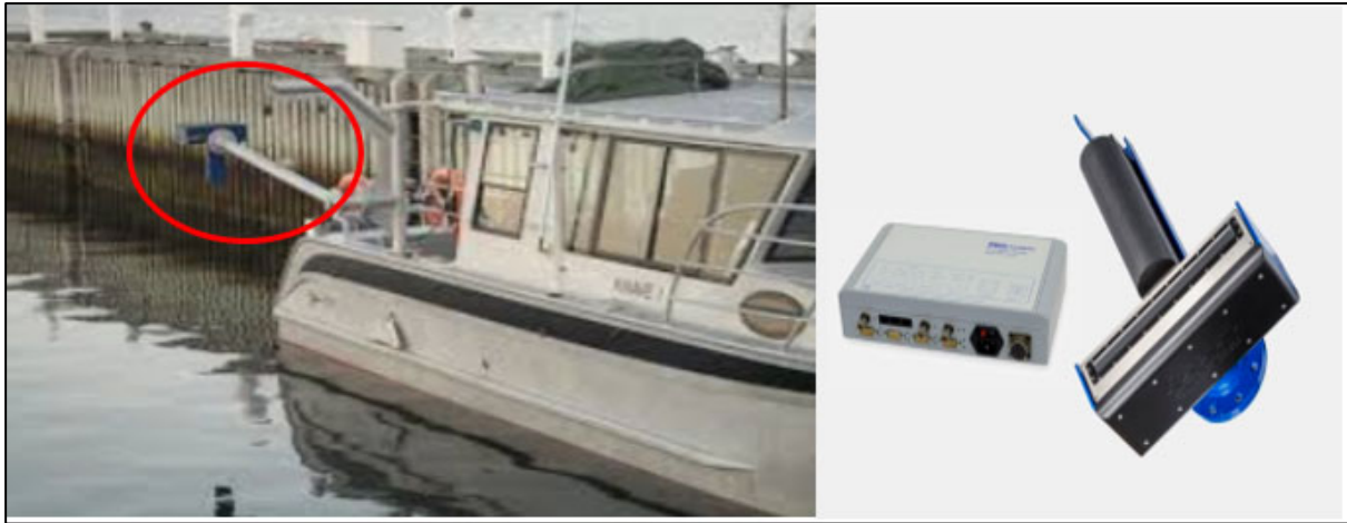
Figure 3: MBES R2Sonic 2024 typical configuration and equipment
