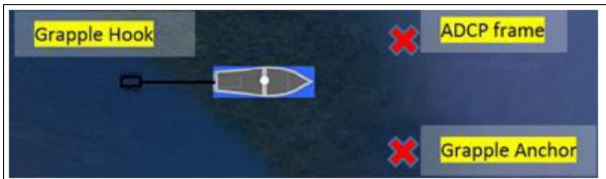
Figure 20: Grapple recovery method (Techworks Marine Ltd)
