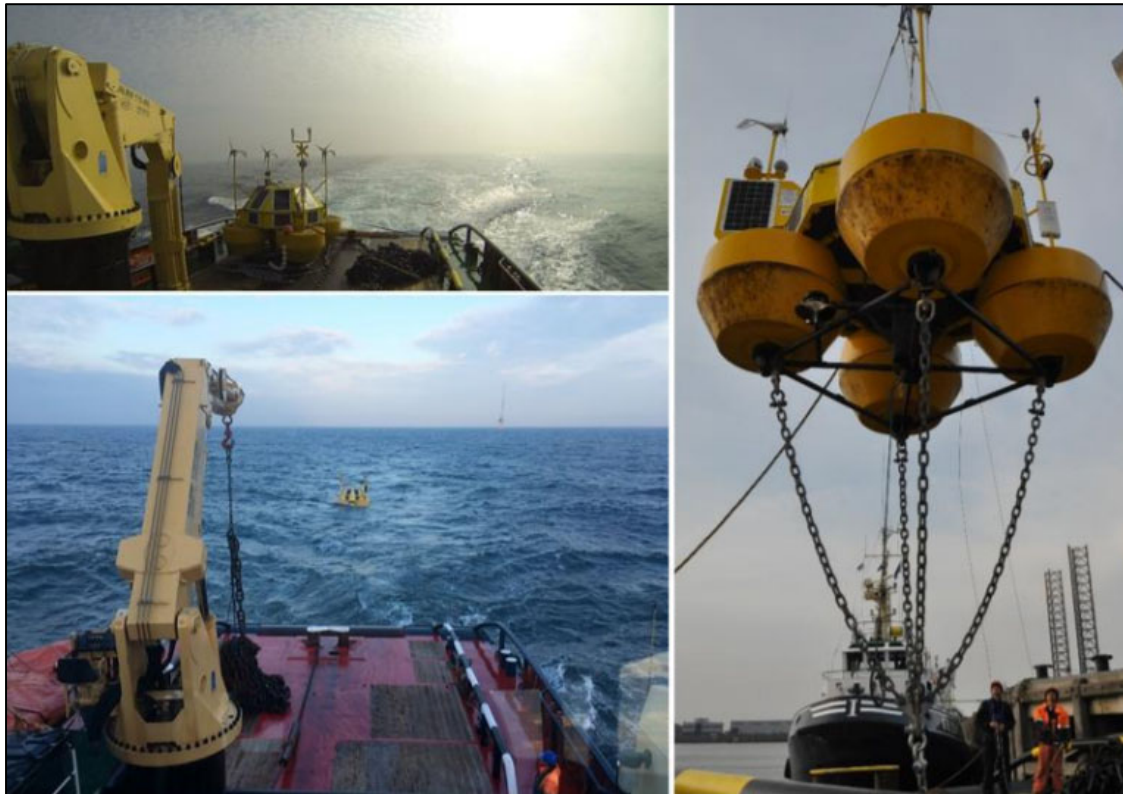
Figure 25: Top left: Lifting down installation option, Eolos FLS200 + mooring on vessel deck; Bottom left: Eolos FLS200 towing operation; Right: Eolos FLS200 lifting to vessel deck with upper mooring
