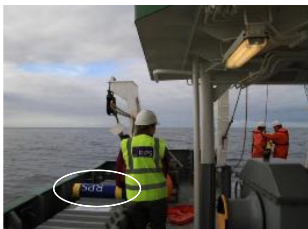
Figure 2.13 Deployment of static underwater acoustic recorders
