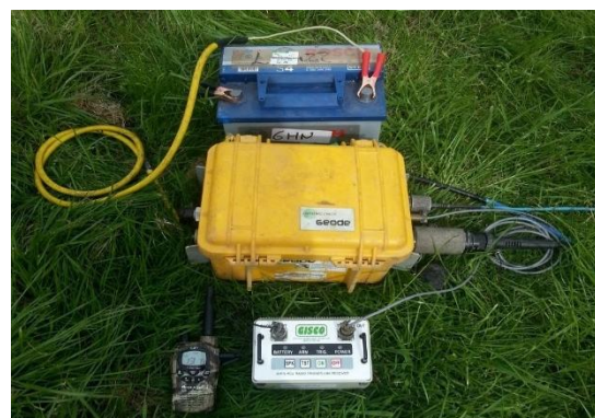
Figure 2.10 Geometrics Geode Seismograph
