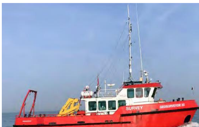
Figure 2.3 Typical offshore geophysical survey vessel (GeoSurveyor XI Call Sign; ORVI)
