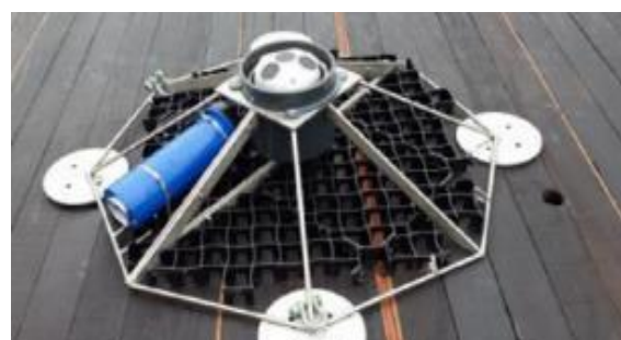
Figure 2.15 Typical seabed frame with ADCP (Ocean Scientific International Ltd)
