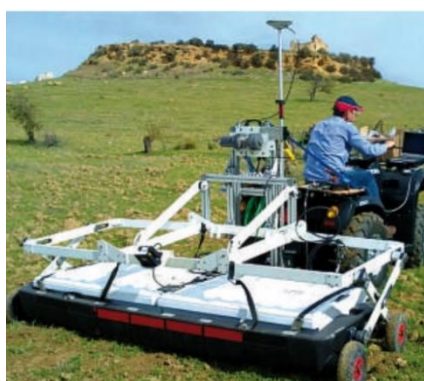
Figure 2.12 Stream X Towed GPR System
