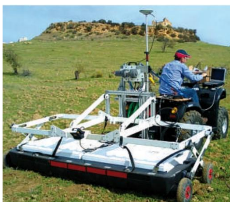
Figure 2-12 Stream X Towed GPR System
