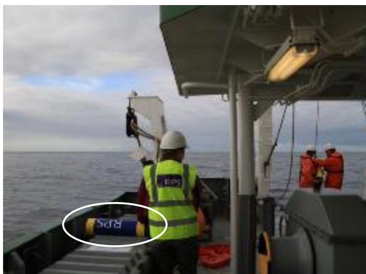
Figure 2-13 Deployment of static underwater acoustic recorders
