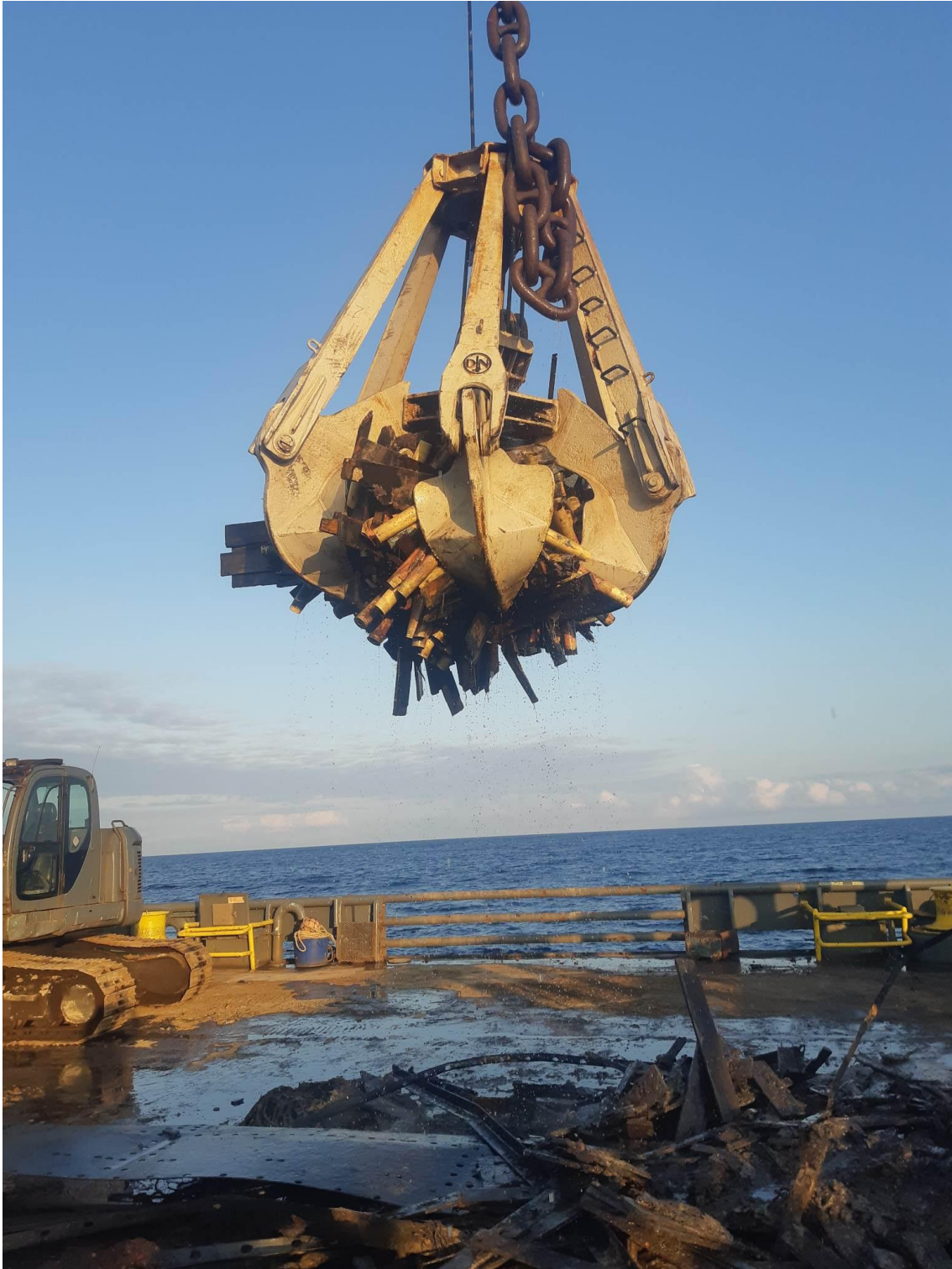
Figure B2. Recovery grab returning repetitive tubular cargo from the target wreck.
