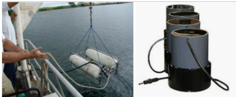
Figure 2-12 Left - Applied Acoustics AA300 being deployed & Right - Typical Hull Mounted SBP - Edgetech 3300
