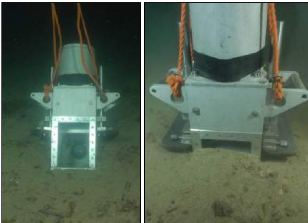
Figure 2-2: Diver operated Sediment Profile Imaging camera. The left-hand image gives a view of the camera at the sediment surface. The right-hand image shows the SPI camera when inserted into the sediment.
