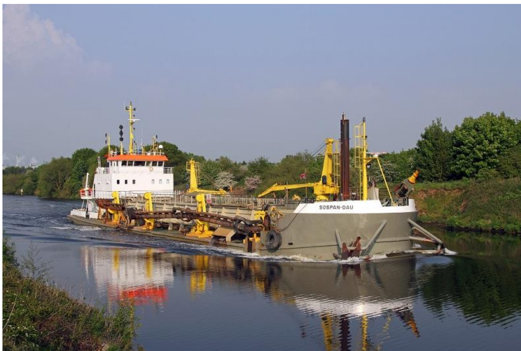
Figure 2-1 Example of Trailing Suction Hopper Dredger (© Sosban BV, 2023)
