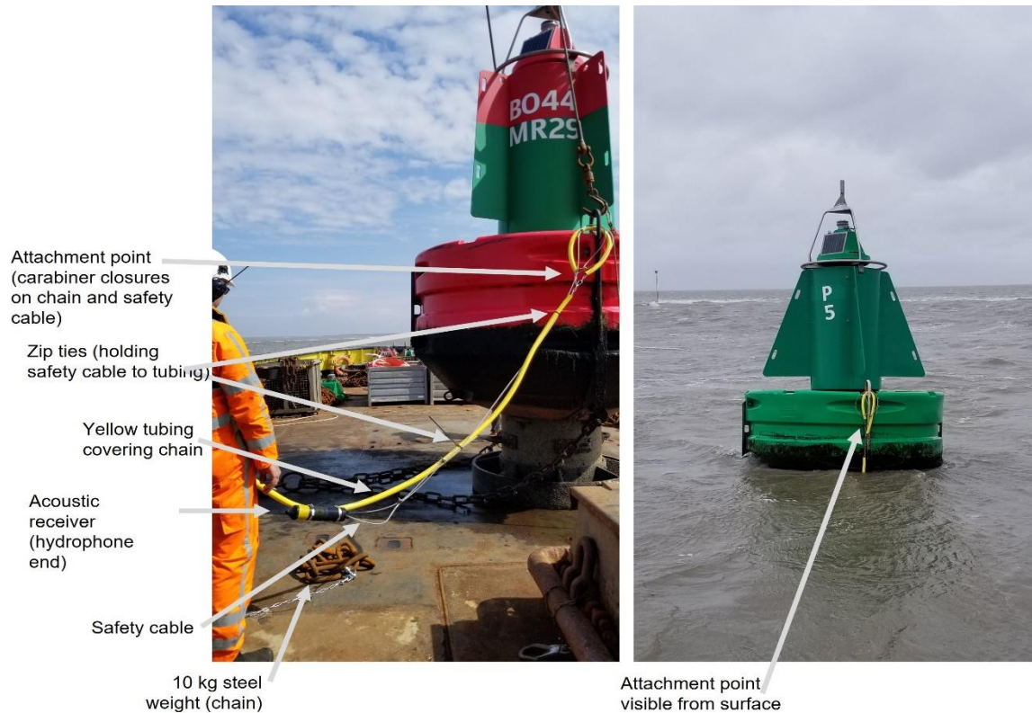
Figure 3. An example of two co-deployed receivers within the Dutch Wadden Sea Swimway acoustic array, shown pre- (left panel) and post- (right panel) deployment. Thirty receivers are currently deployed on the larger buoys (left). Photos provided by [REDACTED]
