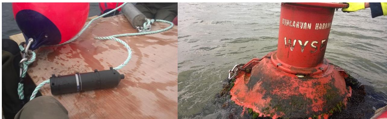
Figure 4. An acoustic receiver deployed on a 14mm polypropylene rope (left) attached using a D shackle through a metal eyelet on a tethered line (right)
