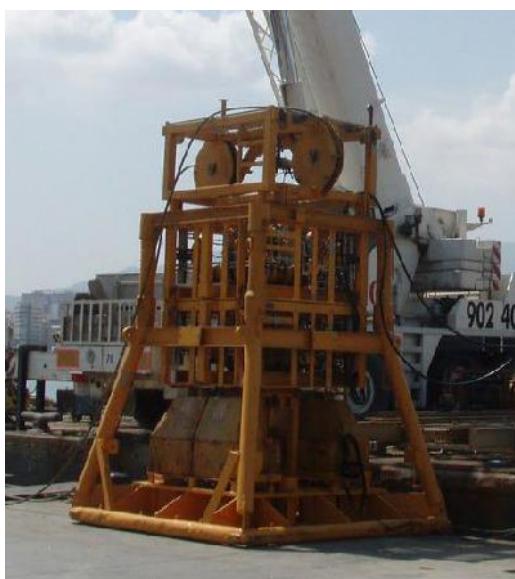
Figure 8-1: Example of a Block Push Seabed CPT System (Fugro Seacalf)
