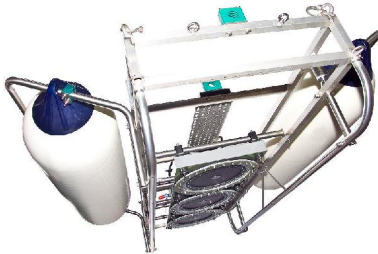
Figure 4: Example of Boomer Sub-Bottom Profiler (INFOMAR, 2023)
