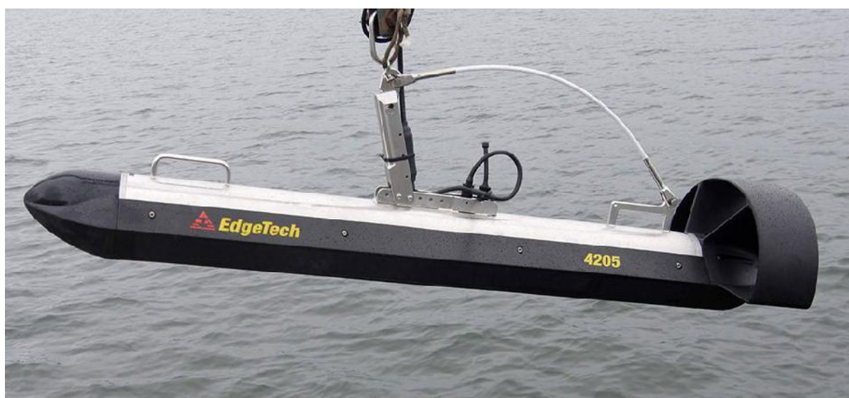
Figure 2: EdgeTech 4205 MP Side Scan Sonar Towfish (EdgeTech)
