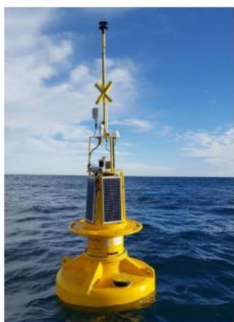
Figure 021: Typical Floating LiDAR (AXYS Technologies)
