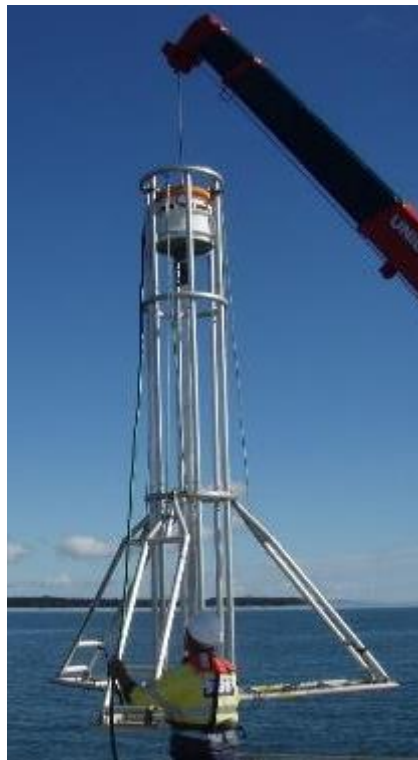
Figure 8-2: Example of a Crane Deployed Vibrocore System
