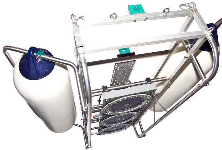
Figure A-0-6: Example of Boomer Sub-Bottom Profiler (INFOMAR, 2023)
