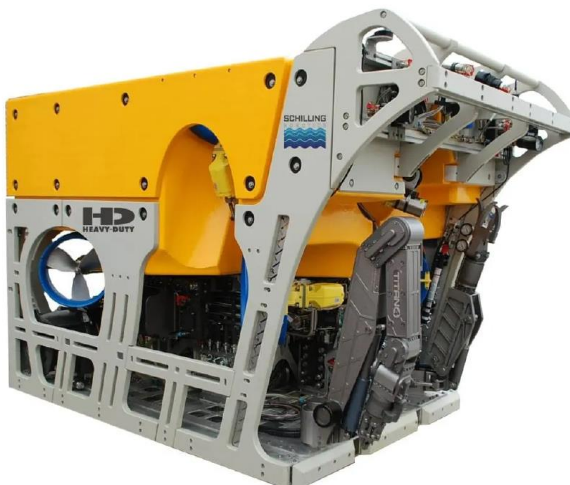
Figure A-0-9: Example of Work Class ROV (Schilling Robotics)
