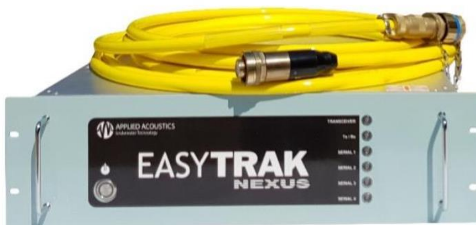
Figure A-0-10: EasyTrak Nexus EZT-2691 topside processing unit (Applied Acoustics, 2023)
