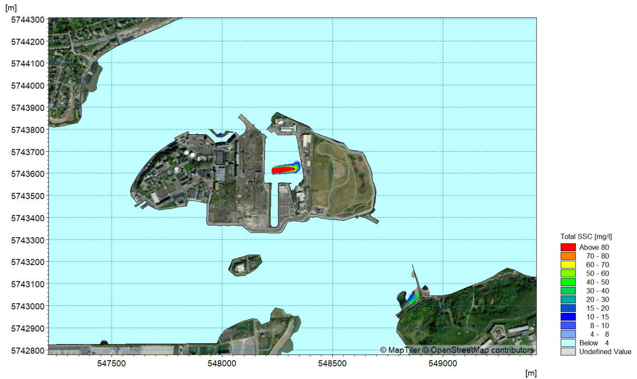
Figure 4.2: Sediment plume envelope created at Low Water from dredging operations in Haulbowline Harbour
