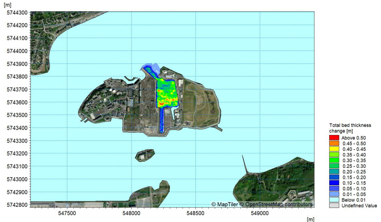
Figure 4.9: Total bed thickness change within Haulbowline Harbour following the proposed dredging operations
