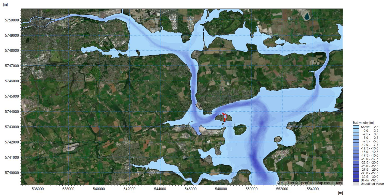
Figure 3.2: Extent and bathymetry of the inner Cork Harbour model
