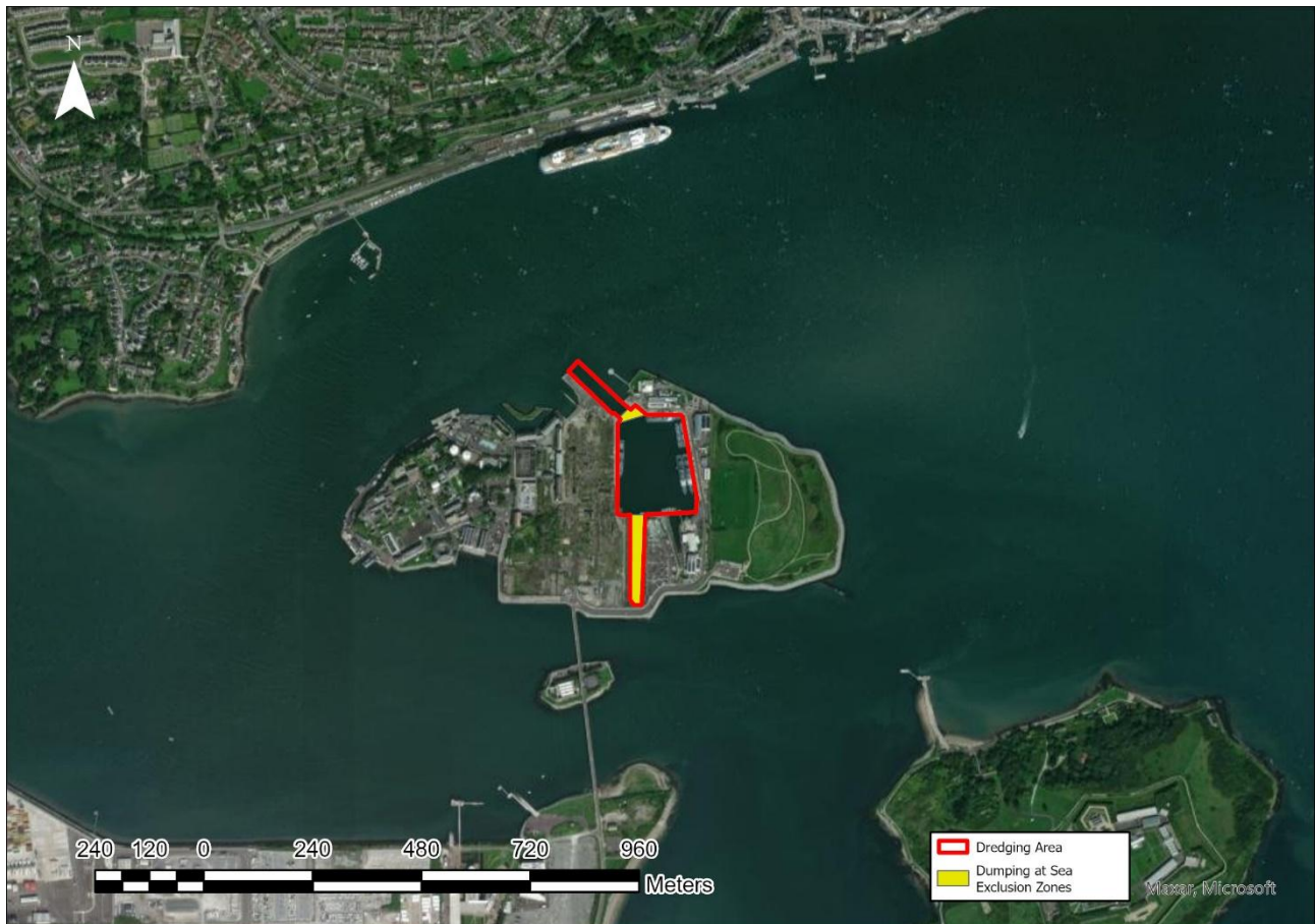
Figure 2.1: Location of the proposed dredging location within at Haulbowline Harbour. The areas to be dredged but not dumped at sea are highlighted in yellow.
