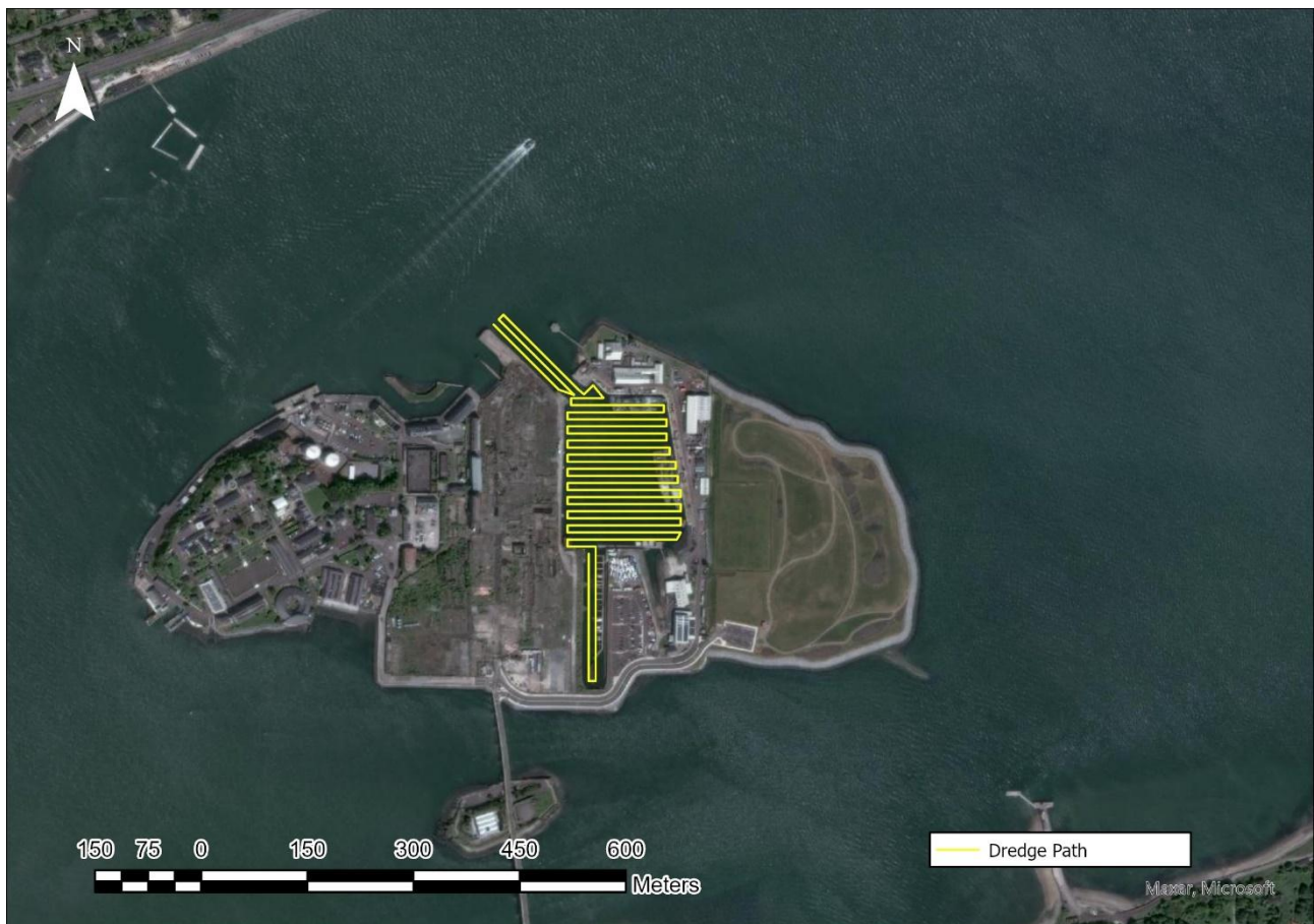
Figure 4.1: The path used to define the location and movement of the dredging source term
