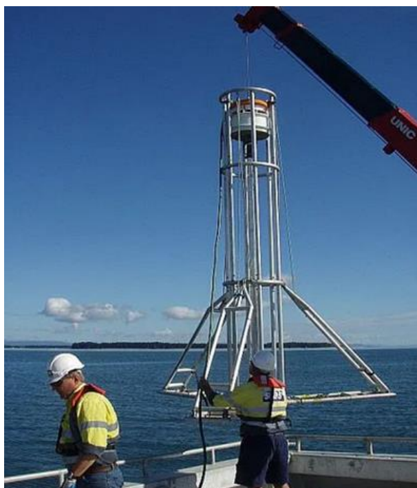
Figure 2.16 Method of Vibrocore Assembly
