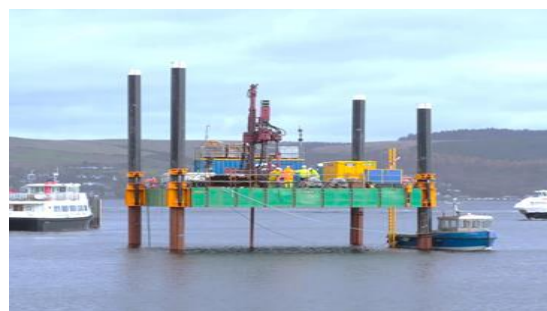
Figure 2.16 Jack-up Barge and drill rig
