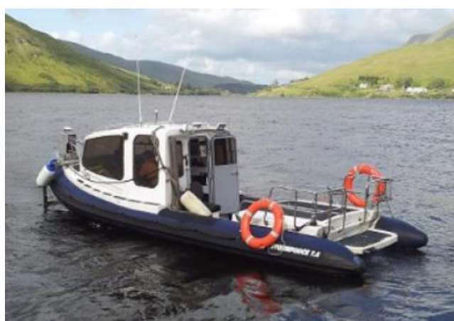
Figure 2.4 Typical nearshore geophysical survey vessel (RV GEO)
