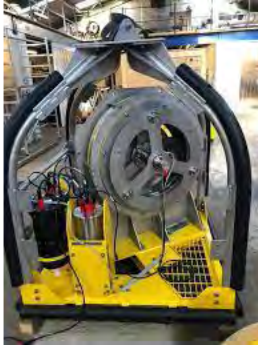
Figure 25. Neptune 3000 CPT rig
