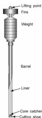
Figure 26. Gravity Corer schematic
